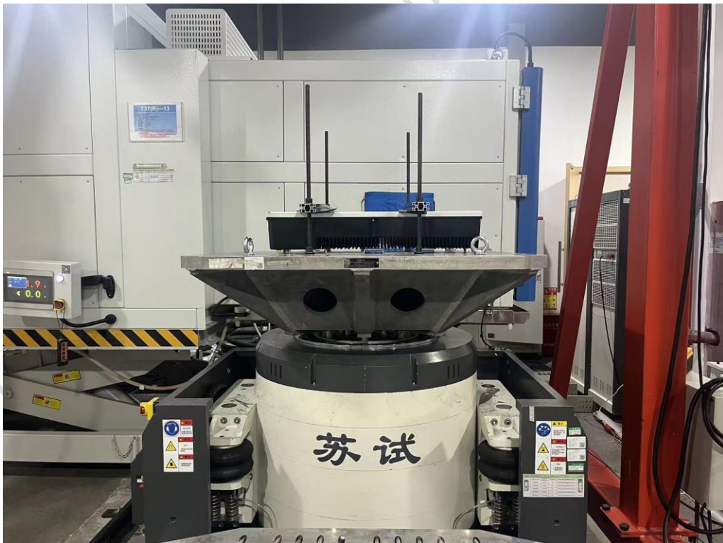
Fixed photos of Z-axis Sinusoidal vibration (bare machine) Random vibration (bare machine) vibration
