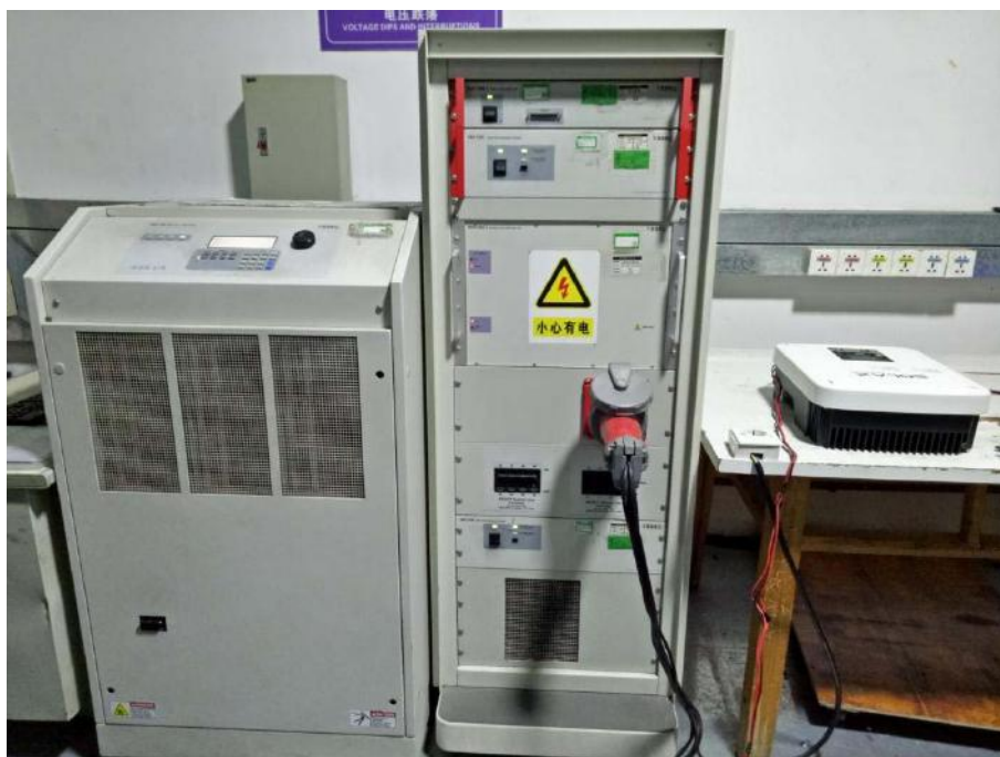
16.10.Photo of Voltage Dips and Interruption Immunity Test
