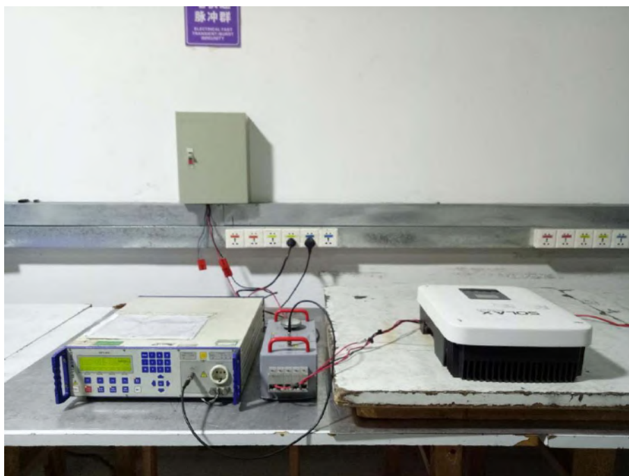
16.6.Photo of Electrical Fast Transient / Burst Test
